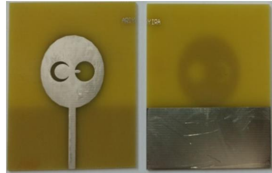
Fig. (18) Fabricated prototype of EMSA with slots in patch
