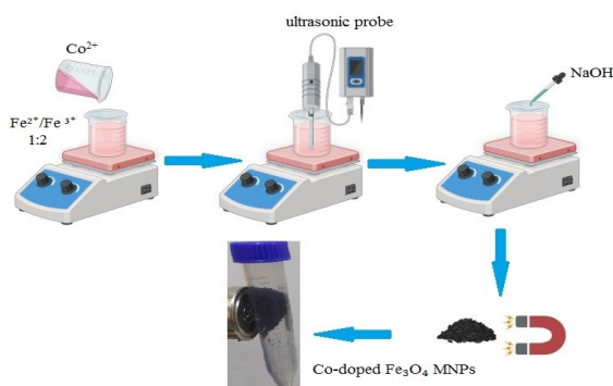
Fig. (1) Scheme of synthesis Co-doped \text{Fe}_3\text{O}_4 MNPs using sonochemical co-precipitation method
