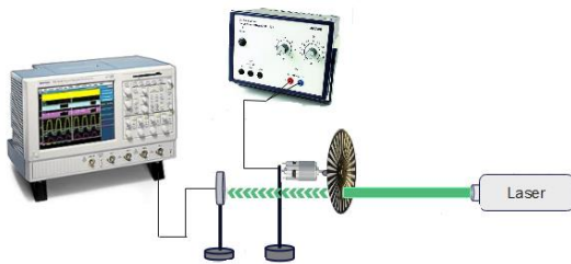
Fig. (1) Experimental setup for Q-switched diode laser using optical chopper
