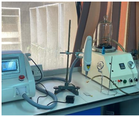
(b) Fig. (8) Sample bombardment by Nd:YAG laser
