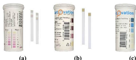
Fig. (3) (a) The strips used (nitrite 0–25 ppm, nitrate 0–500 ppm), (b) Hydrogen peroxide \text{H}_2\text{O}_2 test strips low level [0–100 ppm]), (c) Hydrogen peroxide \text{H}_2\text{O}_2 test strips high level [100–400 ppm])
