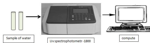
Fig (1) Scheme of UV-visible spectrophotometry carried out on the water samples
