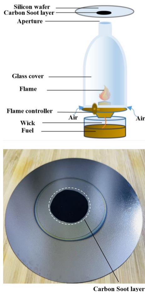
Fig. (1) Production of carbon soot layer on a silicon wafer (a) a silicon wafer is held in the flame for 2 min; (b) a carbon soot layer deposited on silicon wafer
