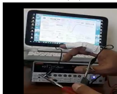
Fig. (5) (A) Electrical conductivity and sheet resistance of the paper based sample, (B) time dependence of the paper based sensor and (C) strain sensor under test
