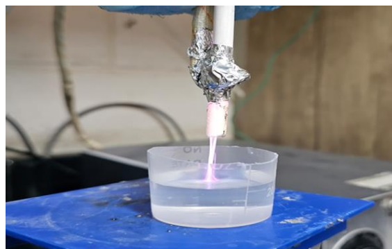
Fig. (2) Plasma system while working to activate the water at Ar gas flow rate of 2.5 L/m
