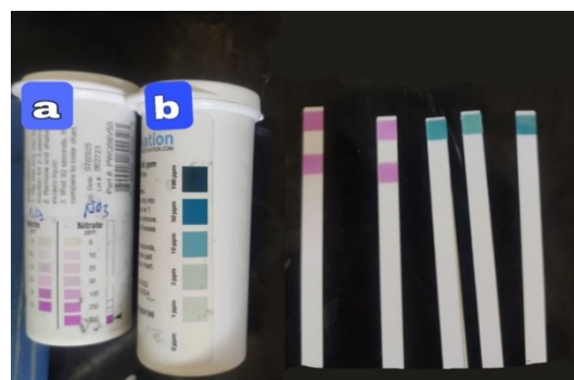
Fig. (3) (a) Test strips for nitrite and nitrate detection (ppm) (b) Hydrogen peroxide test strips (ppm)
