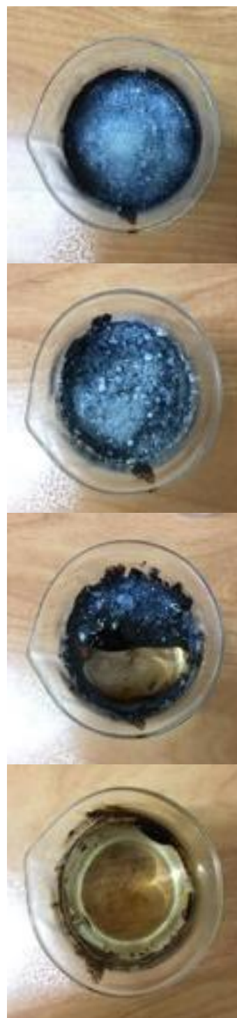
Fig. (10) Photographs before and after the absorption of crude oil by the hydrophobic aerogel
