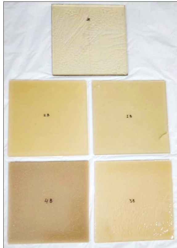
Fig. (S5) Acoustic insulation test specimens. This figure includes the square panels of UPE/HDPE composites labeled Z (0%), 1B (2.5%), 2B (5%), 3B (7.5%), and 4B (10%). These were installed as barriers in the acoustic test rig to quantify reductions in sound pressure levels at 100 Hz, 1000 Hz, and 10,000 Hz. The visual consistency supports the validity of the acoustic data reported in the main text
