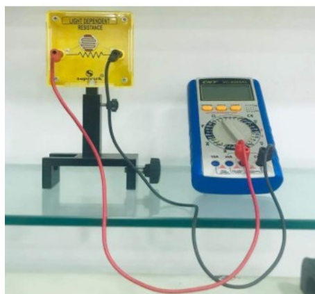
Fig. (1) Circuit used to measure light dependent resistor (LDR)
