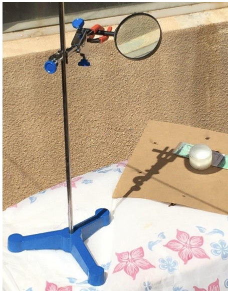
Fig. (1) Photochemical etching system of this work using sunlight as a light source
