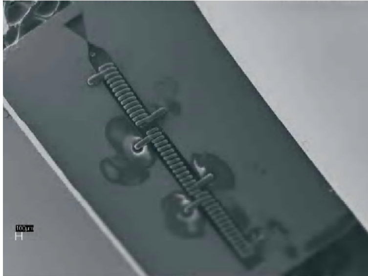
Figure 5.1: Cold/hot gas microthruster etched in silicon with three LCVD-deposited carbon microcoil heaters..
