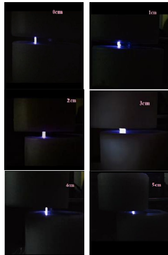
Fig. (3) Influence of horizontal distance on the micro-discharge that formed in DBD actuator in the Presence of the magnetic field
