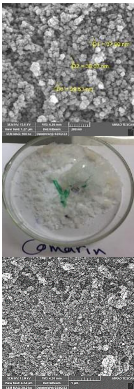
(d) Coumarin density 0.20 \text{ g/cm}^3 Fig. (9) FE-SEM images of doped silica aerogel with (a) copper chloride, (b) silver chloride, (c) fluorescein, and (d) Coumarin with different magnifications
