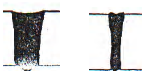
Sample (1) Sample (3) Fig. (3) Cross-section of real laser welds
