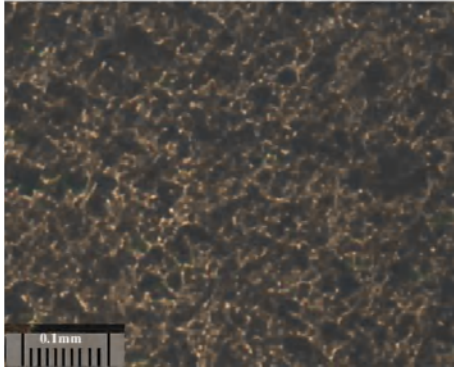
Fig. (2) Microstructure of graphite before attempting the hot uniaxial pressing
