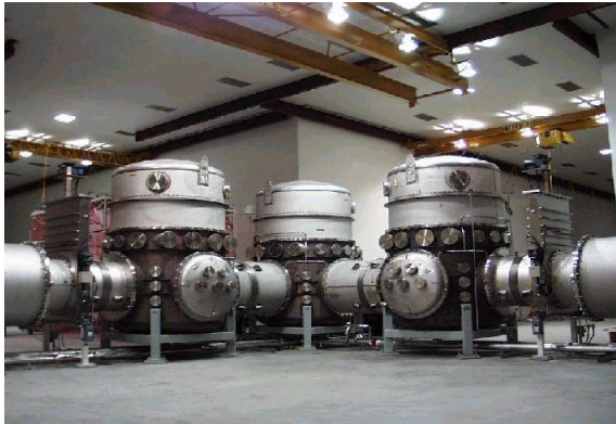
Fig. (19) A photograph of the large vacuum chambers containing the various LIGO detector components is shown. These chambers are isolated from the long vacuum pipes by gate valves to access the equipment.
