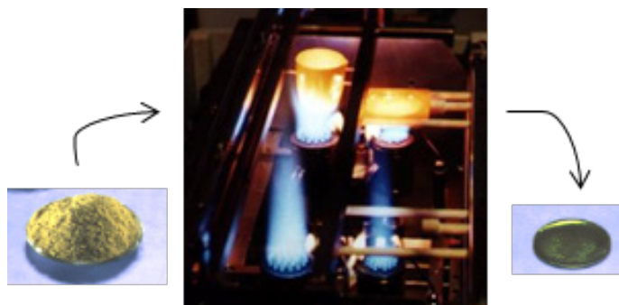
Figure 2: Transformation of the powder material into a glassy sample by fusion at high temperature.
