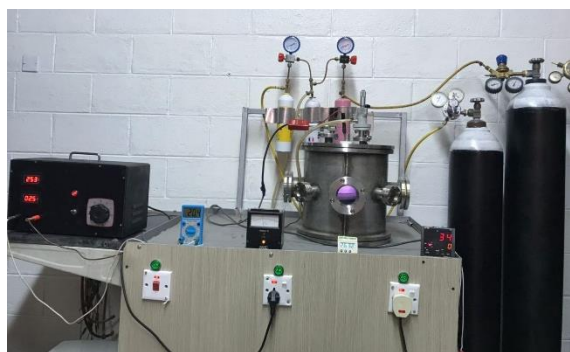
Fig. (1) A photograph of the dc reactive magnetron sputtering system used in this work
