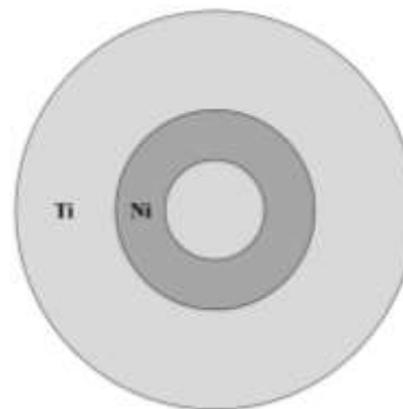
Fig. (2) Geometrical arrangement of the co-sputtering configuration using Ti and Ni targets
