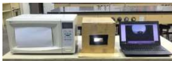
Fig. (3) Experimental setup of contact angle measurement
