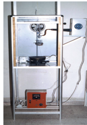
Fig. (1): Spray pyrolysis system used to grow CdS:Ag layer
