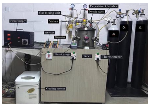
Fig. (1) A photograph of the dc reactive magnetron sputtering system used in this work
