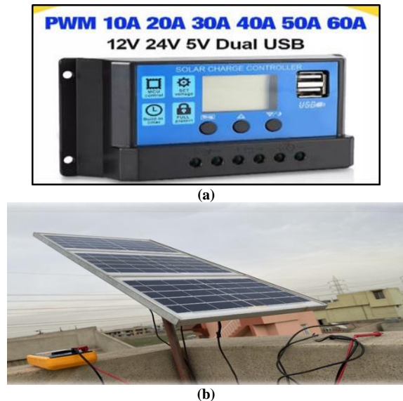
Fig. (1) System configuration (a) charging regulator, and (b) solar panels
