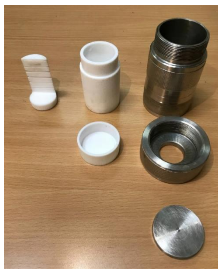
Fig. (1) Autoclave and Teflon rack used to deposit CuO thin film hydrothermally on FTO substrate
