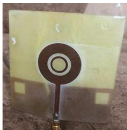
Fig. (11) Fabricated prototype of CCMA with slots
