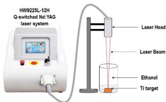
Fig. (1) Schematic diagram of PLAL setup used in this work
