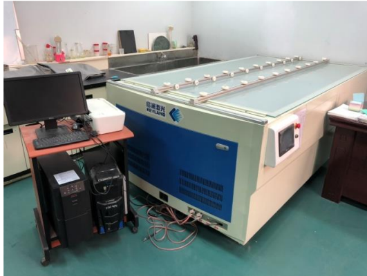
Fig. (1) The Keyland Photovoltaic Sun Light Simulator used for STC test
