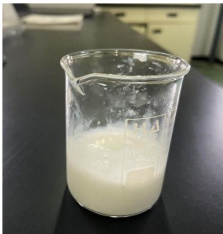
Fig. (2) The solution of the paint after 5 min probe sonicating
