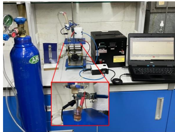
Fig. (1) Configuration of non-thermal plasma jets system, spectrometer, and electronic controller
